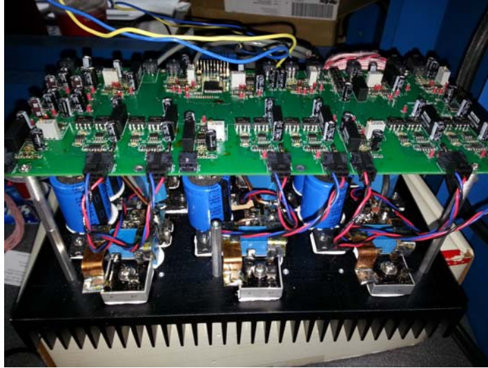
Figure 3. Laboratory prototype of a 3-phase PFC rectifier as constructed in NYU-Poly power laboratory.
